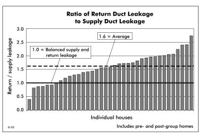
On average, return ducts were responsible for 60% more leakage than supply ducts—not surprising since much of the return system relies on building cavities. The excess of return duct leakage raised concerns about depressurized basements and combustion safety.
