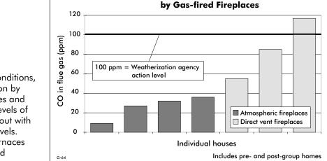
Under normal operating conditions, carbon monoxide production by most water heaters, furnaces and fireplaces was well below levels of concern. A few units stood out with higher carbon monoxide levels. Note that water heaters, furnaces and fireplaces are all vented to outdoors.
