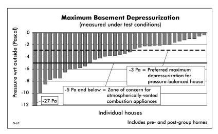
Under test conditions, all basements were depressurized with respect to outdoors. These negative pressures were of the same order of magnitude as the measured draft pressures in water heater and furnace flues, raising concerns about the abilities of these appliances to successfully remove combustion products from the house.
