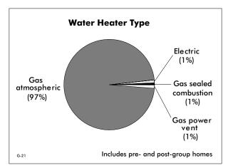
Gas-fired, atmospheric water heaters were the norm, raising concerns about combustion safety.
