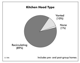
Few homes had vented hoods, even when gas ovens were present. A recirculating range hood coupled with an over-the-stove microwave oven was typical. This type of hood provided some degree of filtration but did not exhaust pollutants outdoors.
