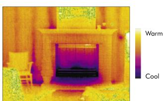
The owners of this house complained about drafts that made their living room uncomfortably cold. The infrared photo (right) shows the cold air that leaked around the fireplace unit. (This was a direct-vent fireplace, so there were no leaks between the room and the vent; all leakage was due to an incomplete air barrier in the cavity enclosing the unit.)
