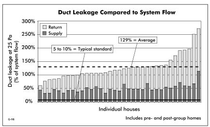
Comparison of air flows at registers versus the flow through the air handler provided further evidence of the magnitude of duct leakage.
