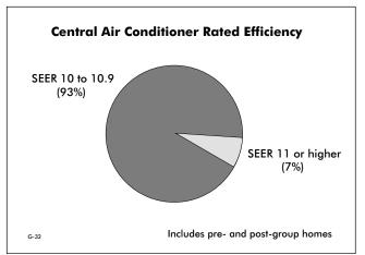
Most heating and cooling equipment was rated at or slightly above the federal minimum efficiency standards referenced by the energy code. Almost all furnaces were rated at 80% AFUE, versus a minimum standard at 78% AFUE (Annual Fuel Utilization Efficiency, the seasonal efficiency rating). Almost all air conditioning units were rated between 10.0 and 10.9 SEER, versus a minimum standard of 10.0 SEER (Seasonal Energy Efficiency Rating).
