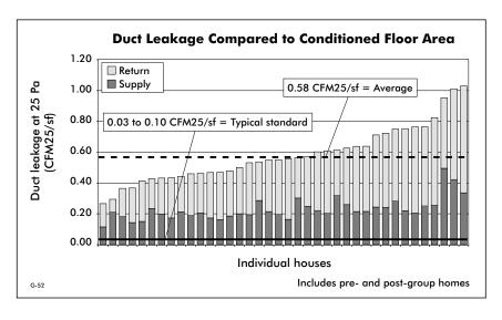
These graphs show measured duct leakage in absolute units (top), leakage compared to the size of the house (middle) and leakage compared with system air flow (bottom). Standards used elsewhere are shown for reference.
