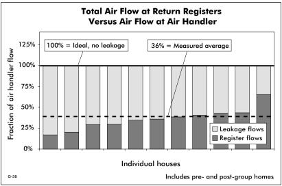
In a subset of homes, air flows were measured at each register. The total of the individual register flows was compared with the measured flow through the air handler. On average, about 80% of the flow through the air handler reached supply registers, while only about one-third of the air handler flow was drawn from return registers (the balances were made up via leakage).
