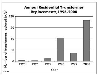
Larger homes and the increasing prevalence of residential air conditioning have caused the need to replace many distribution transformers since 1998. In response, Fort Collins Utilities increased transformer sizing criteria in 2001.
