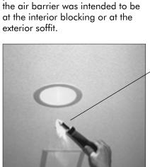
large amounts of air leaking through recessed lighting located in floors with heated space above and below. This could be a symptom of leaks in the air barrier at an exterior cantilever: air moved through the floor joist cavities to exit at the light cans.
