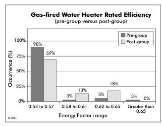
The seasonal efficiency of a water heater is rated as an "Energy Factor" from zero to 1.0 (0% to 100%). The majority of study home water heaters had Energy Factors at or just above the federal minimum standards referenced in the energy code. However, the trend from pre- to post-group homes showed an increase in the use of higher efficiency units.
