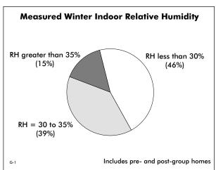
Dry indoor air during the winter was a common comfort complaint, borne out by humidity measurements.
