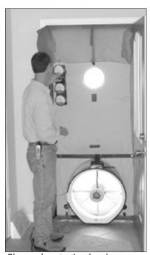
Blower door testing has been increasingly used to document compliance with the code's air sealing requirements.
