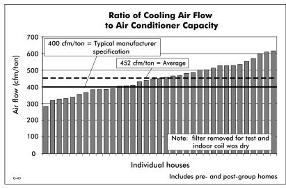
In about half of the air conditioning units, measured air flow across the indoor coil deviated considerably from manufacturer specifications. Low air flows reduce equipment efficiency and capacity. Excessively high flows use more fan energy than necessary for design performance.
