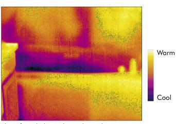
The infrared photo above shows the symptom of a missing air barrier: a cold tub. This bathtub sat against two exterior walls and over a garage. Cold outdoor air moved through or around the insulation to cool the tub. (Infrared photo taken with blower door operating.)
