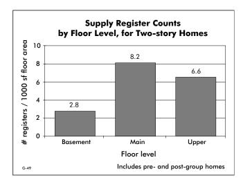
Upper levels had fewer supply registers per square foot than main levels, presumably because of the challenges of running ducts to upper level rooms. The paradox: upper level rooms had higher heating and cooling loads per square foot than main level rooms. (Basements typically had the smallest number of registers because many study home basements were unfinished and not intentionally conditioned).
