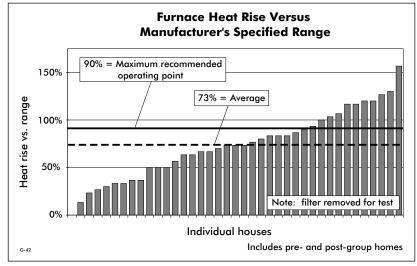
About one-quarter of the furnaces operated at or outside manufacturer limits for "heat rise." High heat rise indicates low air flow or overfiring. It reduces efficiency and reduces equipment lifetime by putting more thermal stress on the heat exchanger. Low heat rise may mean the air delivered to the house is too cool for comfort.
