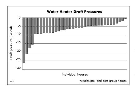
The buoyant force that pulls combustion products out of the house via the flue is called the "draft pressure." Measured draft pressures in water heater and furnace flues were very small; the 0-to-10 Pascal range was typical.
