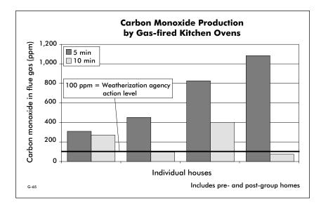
Carbon monoxide production by gas ovens was highest in the first few minutes of operation. After the burner had been on for 10 minutes, carbon monoxide levels had dropped significantly yet remained high enough to be a concern in three of four units. Note that all combustion products from gas ovens were exhausted into the houses and that only one in 11 study homes with gas ovens had a vented range hood.
