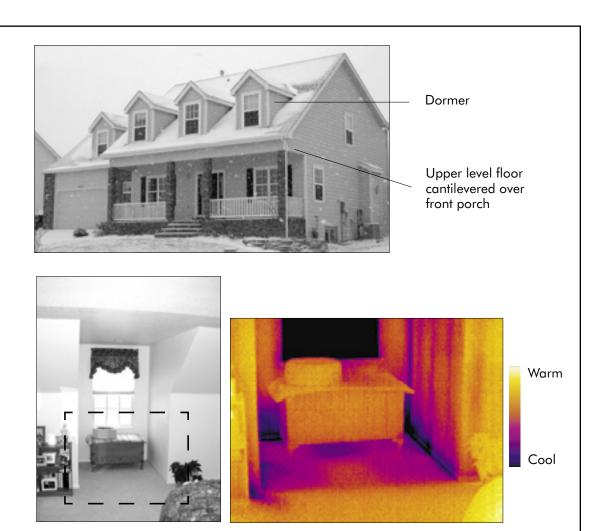
The upper level dormers and cantilever floor in the house shown above posed air sealing and insulation challenges. From the interior (conventional photo lower left, infrared photo lower right), thermal flaws showed up as cold spots (dark). These can cause discomfort and provide opportunities for moisture condensation, mildew and mold growth. The owners of this house complained that the dormers were so cold that they could not use these areas during the winter.
