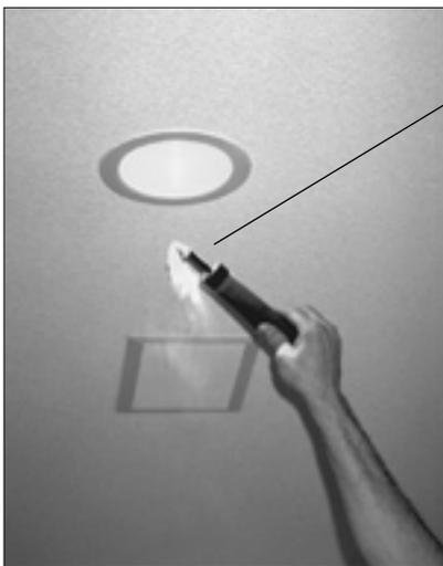
Smoke source made air movement visible.
